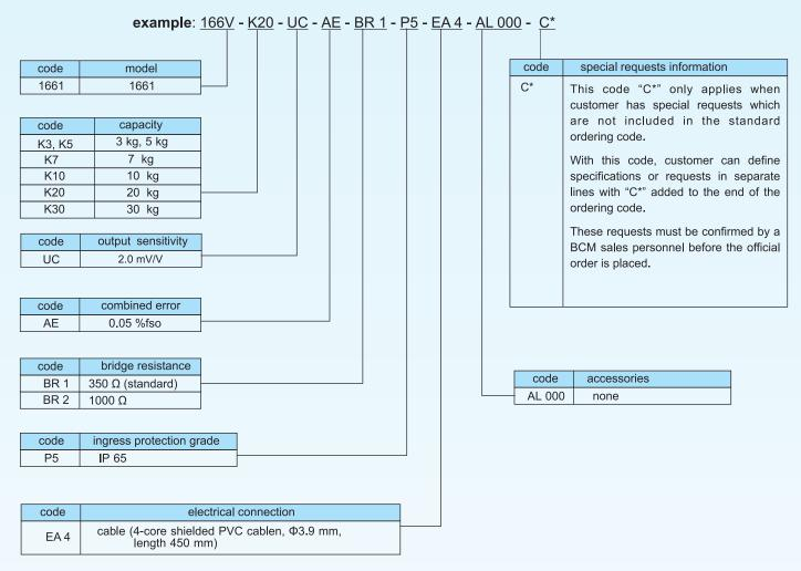
Ordering Code Example: 166V - K20 - UC - AE - BR 1 - P5 - EA 4 - AL 000 - C\* cable length = 500 mm
