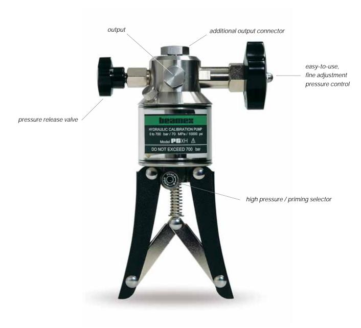
**The PGXH** is a hand-held hydraulic high-pressure generator compatible with many different liquids (e.g. mineral oil, distilled water etc.) A "Skydrol" option is available. The pump is equipped with an adjustable volume control providing fine-tuning of generated pressure. The PGXH can be equipped with an optional relief valve providing adjustable over pressure protection in different ranges.
