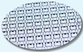
SE107 silicon differential capacitive sensor wafer
