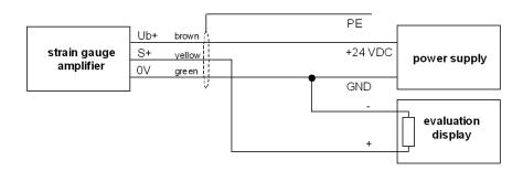
Pin assignment for cable integrated amplifier
