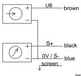
Pin configuration of connector M12x1 (4-pin) /
