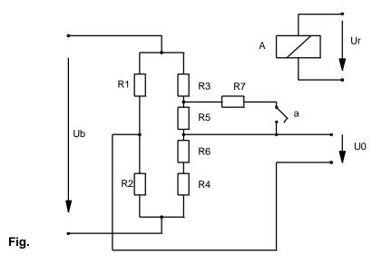
The connection of resistor R7 will always result in a defined unbalancing of the zero point (diagonal voltage) of the Wheatstone Bridge.
