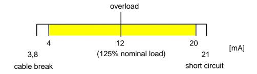
With activating the check relay a fixed signal jump of 8 mA will exceed the overload limit in every working condition. The measurement's upper limit of 20 mA however will never be reached. This makes the checking of the signal jump possible.
