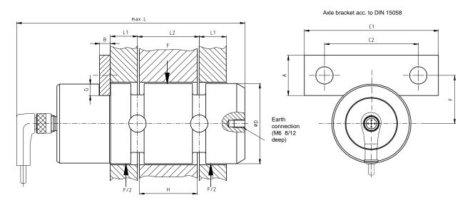
The dimensions for the load pins are according to the customer requirements of the existing bearing.
