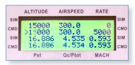
the Hand Held Remote Control, the Touch Screen Remote Control or a wireless Bluetooth connected PDA. All the important air data functions are simultaneously displayed on all interfaces, constant screen or menu changes are not required. Readings of both commanded and measured test values are displayed.
